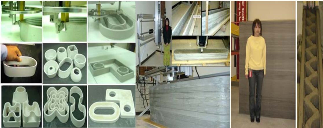
Figure 1 Structures built by Contour Crafting
