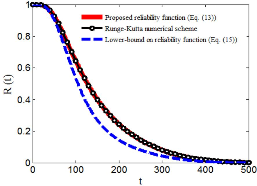
**Figure 2.** A comparison between the subsystem reliability functions obtained from Eq. (13), numerical scheme and the relevant lower-bound
