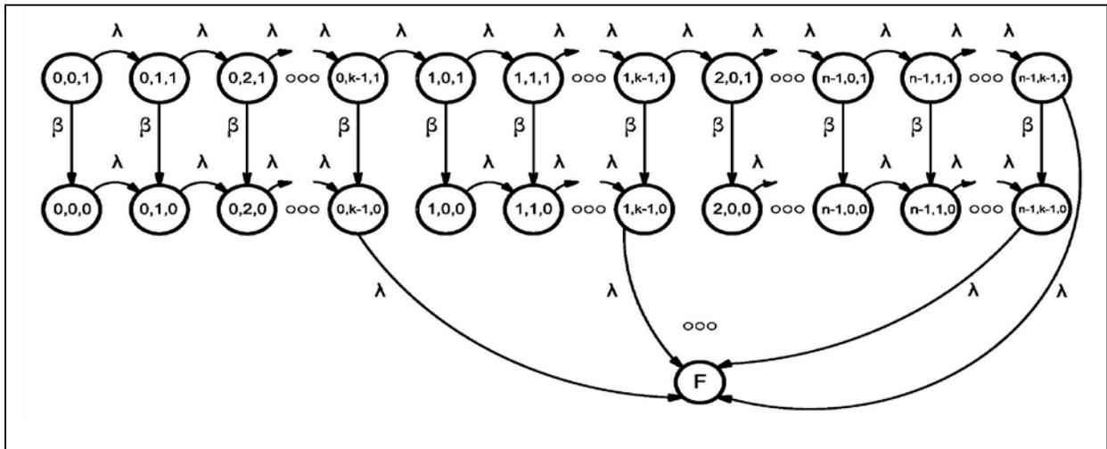
Figure 1. State transition diagram of cold standby subsystem with Case 1 of switching mechanism
