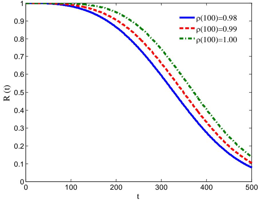
**Figure 6.** The effect of switch reliability on system reliability
