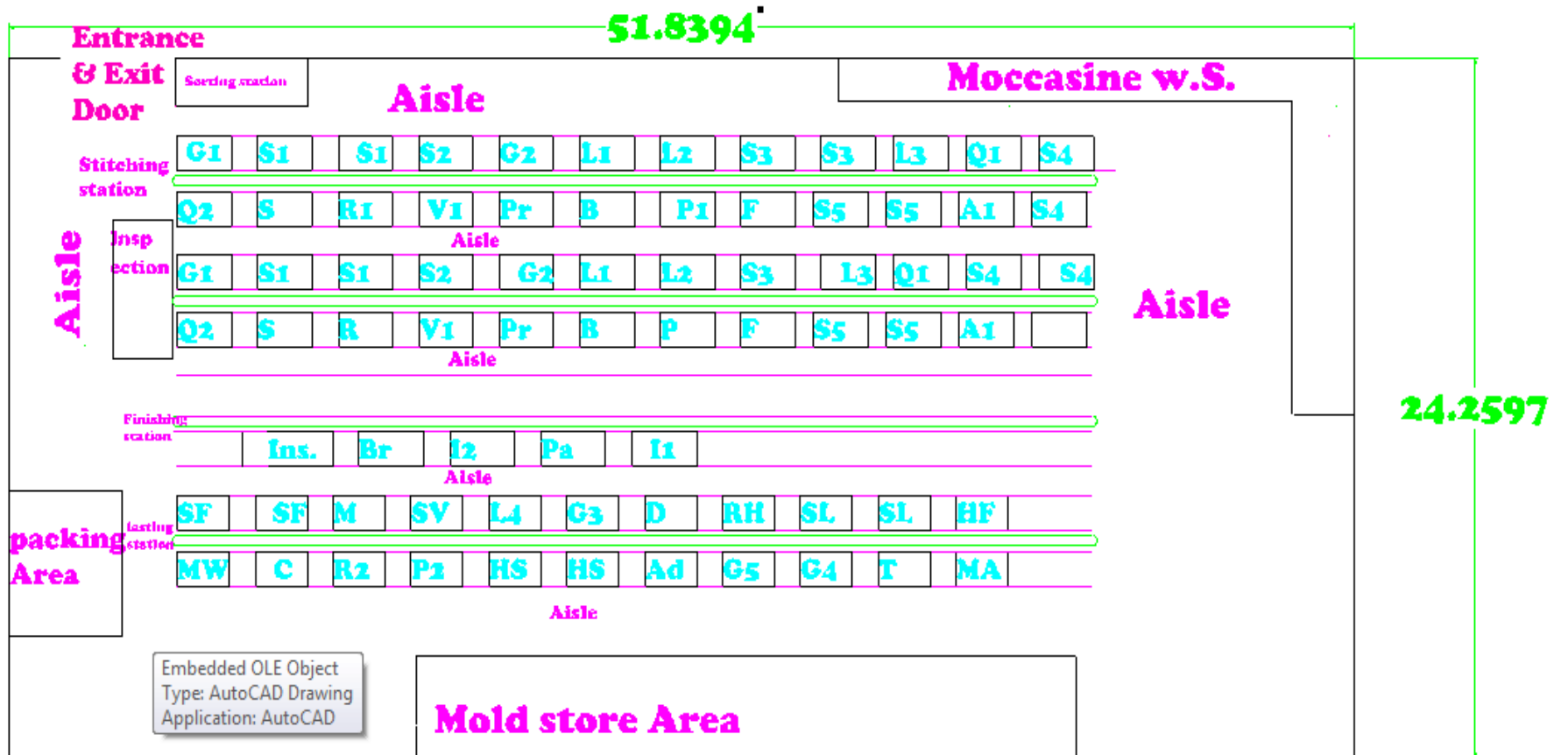
Fig. 9. Existing layout of the stitching, lasting and finishing assembly lines (dimensions are in meter)
