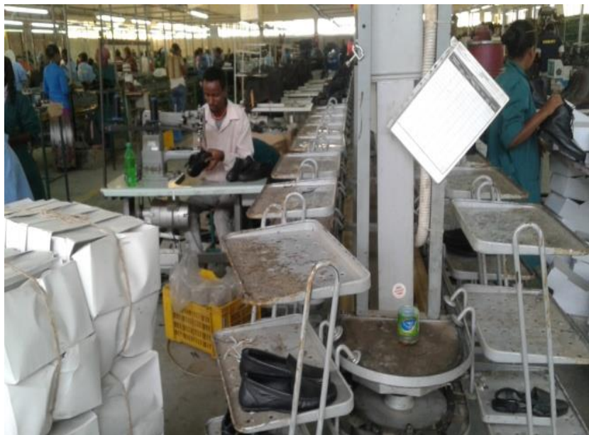
Fig. 2. Lasting and finishing assembly line of Ramsay shoe factory
