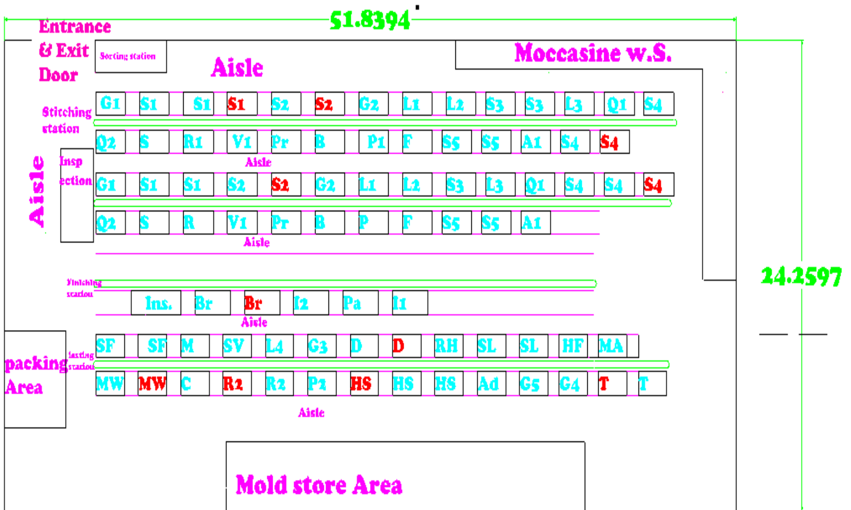
Fig.12. Layout of proposed scenario for three assembly lines (dimensions are in meter)
