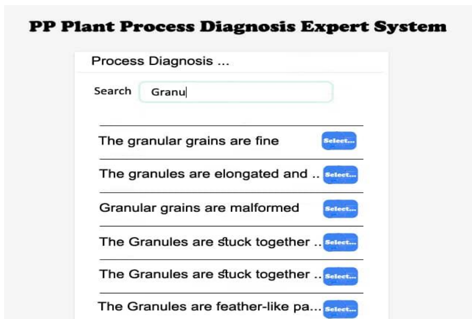
Fig 5. Intelligent system of fault detection in the polypropylene production process
